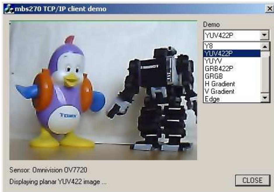
Select an alternate image format from the drop down list in two steps: first select Standby to stop current acquisition then select new format to enable the server to reconfigure image acquisition.
